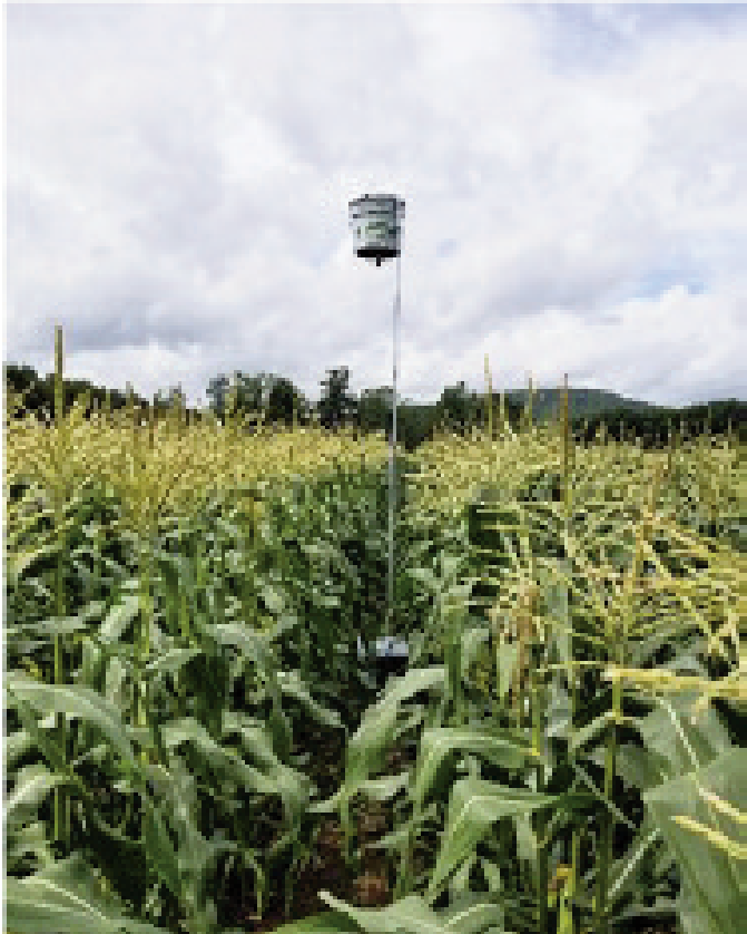
Laser scarecrow unit deployed in a field of sweet corn in Albany County.
